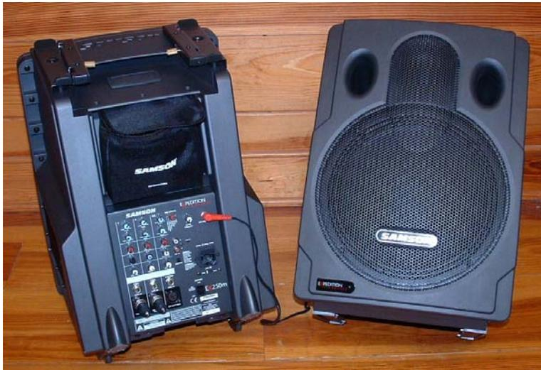
We have invested in some new equipment to better serve our clients. The first is a powerful amplified loudspeaker system that is more easily carried to the field for testing. The Samson Expedition system has the amplifier and some equalization control built into one of the speakers. A second speaker provides the ability to get a more even sound distribution and more reliable test results with a single test when testing isolation between spaces. To provide the noise signal
