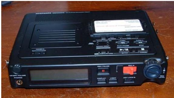
The other new item is a Marantz PMD 671 portable solid state digital recorder. This looks very much like a portable tape recorder, but records digitally directly onto a compact flash memory card similar to those used in digital cameras. It can provide very long recordings at a reduced quality, or the highest possible recording quality for shorter periods with battery power and no moving parts.
